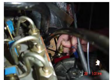
**Note: Secure all fuel lines with cable ties. Cable ties are an economical way to prevent the possibility of problems occurring!**
