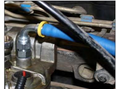
**Note: Secure all fuel lines with cable ties. Cable ties are an economical way to prevent the possibility of problems occurring!**
