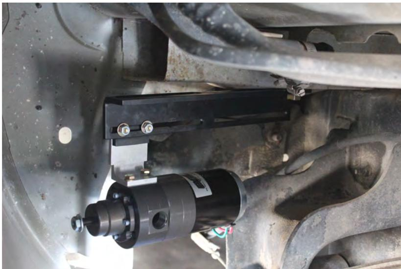
**VERY IMPORTANT: REMEMBERING THE POSITION OF THE "T" PORT, THERE IS A SMALL WEEP HOLE IN THE BASE DIRECTLY NEXT TO THE ELECTRIC MOTOR, THIS HOLE MUST AIM DIRECTLY TO THE GROUND!! IMPROPER INSTALLATION OF THE PUMP CAN CAUSE PREMATURE WEAR AND VOID MANUFACTURES WARRANTY.**
